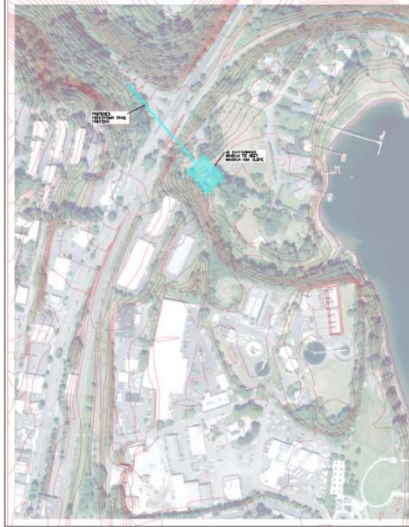
OPTION 2: PEDESTRIAN BRIDGE WITH SWITCH BACKS MEETING MINIMUM ODOT CLEARANCE AND MAXIMUM ADA PEDESTRIAN SLOPES.
