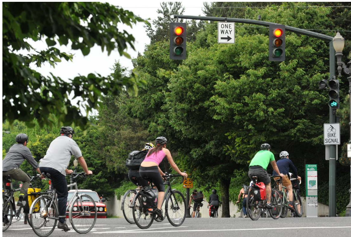
Bicycle signals separate bicycle movements through the intersection, increasing safety. Rose Quarter at the Eastbank Esplanade in Portland.
