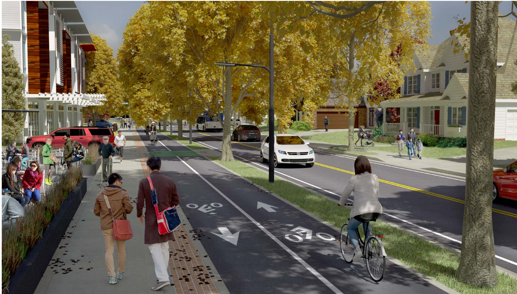
Community street. This rendering illustrates a two-lane minor arterial. The surrounding land use is primarily neighborhood with some small businesses. Buildings are between one and four stories. The separated bikeway provides additional buffer between people on the sidewalk and traffic.
