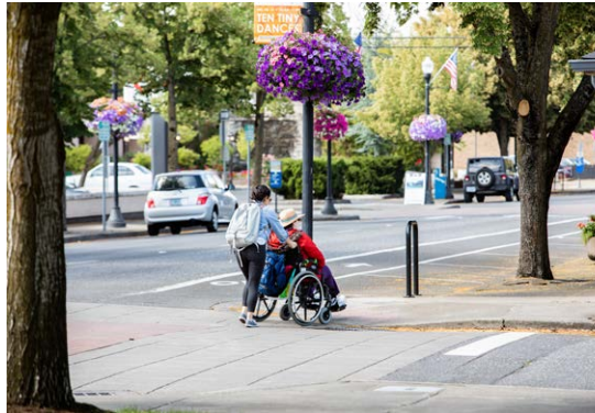
Stop-controlled intersections can provide safe and comfortable spaces for all users in a variety of settings. Marked crossings increase motorist awareness and pedestrian visibility. Raised crosswalk in downtown Beaverton.
