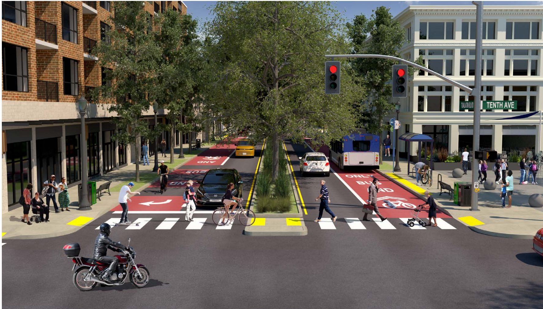
Community boulevard. This rendering illustrates a four-lane arterial in a regional center. Buildings are between two and six stories high. Due to space constraints, a parallel bicycle boulevard provides an alternative route to shared bus-bicycle lanes. Bicycle parking along the street and wayfinding provide access to the street for bicyclists. Due to space constraints, transit riders cross the bikeway to board the bus. A median increases safety.
