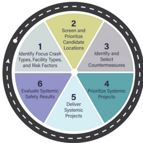
Figure 4: Steps of the Systemic Safety Analysis Source: FHWA, Systemic Safety User Guide , August 2024
